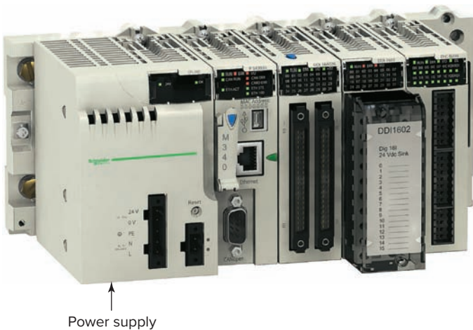
Figure 1-11 The power supply supplies DC power to other modules that plug into the rack. Source: Photo of PLC Modicon M340 © Schneider Electric, 2010. www.schneider-electric.com .
